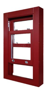
Sash windows English-type function in the sliding system up - down. They are equipped with special weights that support the movement of the wings by a counterweight or a spring.
